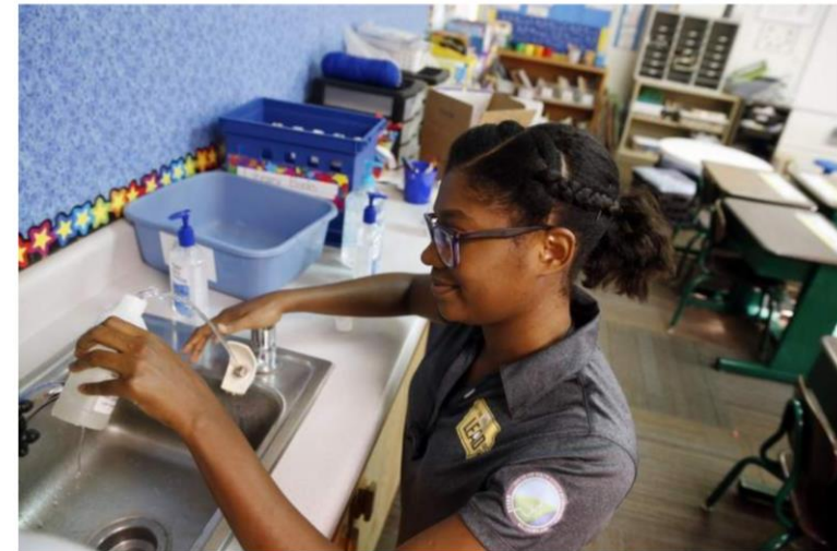
Amina Grant, a third-year Ph.D. environmental engineering student at the University of Iowa, collects a sample from a classroom water fountain during a Nov. 23 retest for lead levels at Strawberry Hill Elementary School in Anamosa on Saturday. All faucets and fountains in the school were tested earlier this year, and the one faucet that tested above federal standards had the pipe and fixture replaced. (Liz Martin/The Gazette)
