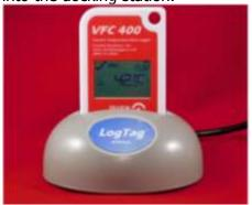
6. After downloading the data from the LogTag, review the data to determine what temperature was reached and the length of the excursion. Complete the Temperature Excursion Checklist.
