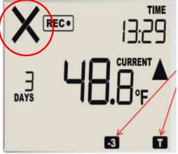
Press and hold the STOP button until "STOPPED" is displayed on the screen (approximately 2 seconds) and the REC symbol disappears. Release the button quickly.
